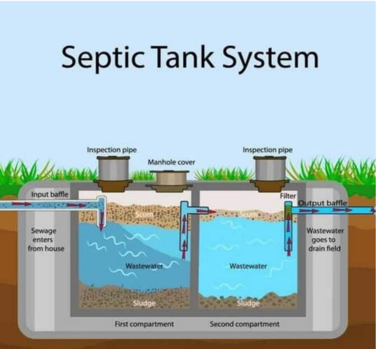
Fig. 4.11, Two Compartment Septic Tank, www.egsd.com/septic-sysyem-types.html
