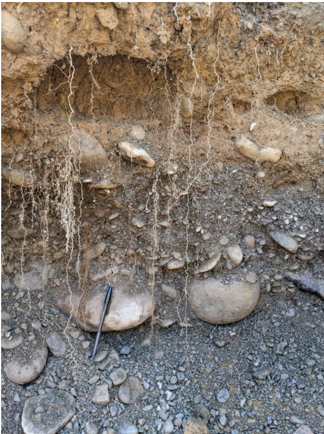
I-6C B-horizon 0-0.5 m silt to cobbles. 0.5 to 0.7 m coarse sand to pebbles. 0.7 to ~1 m coarse sand to cobbles. Layers are approximately horizontal (difficult to measure).
