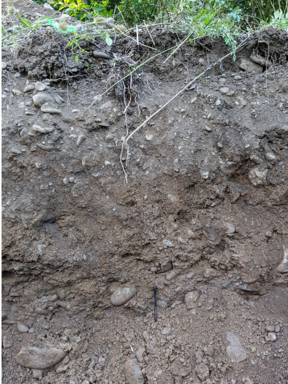
I-6D At north side of pond. The pond is approximately 1.2 m south with some standing water. Medium sand to cobbles. No sedimentary layering. Pebbles and cobbles are matrix supported. Total depth 1.3 m. Moist at bottom.
