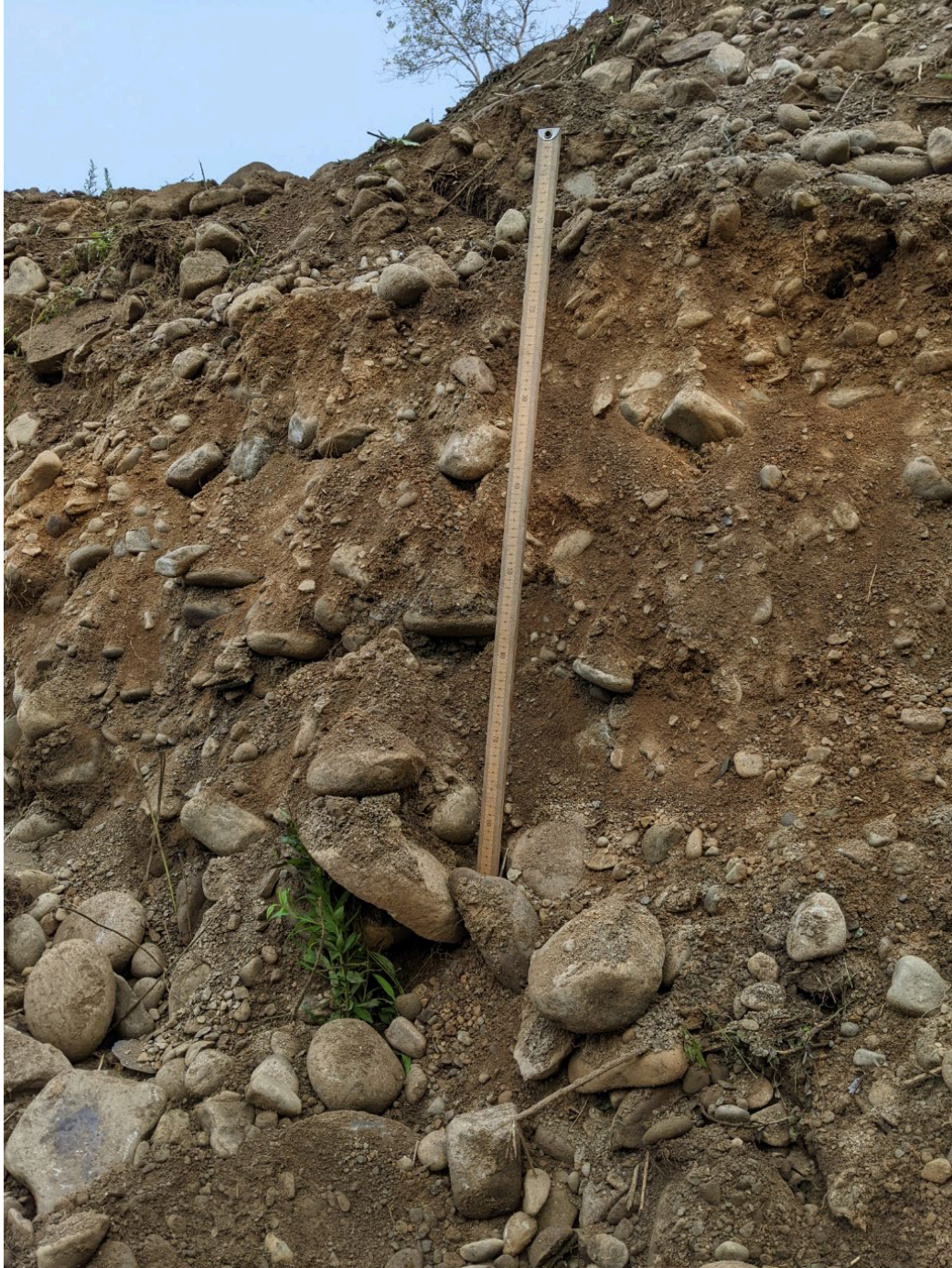
I-4B Medium sand to cobbles. Cobbles are matrix supported.
