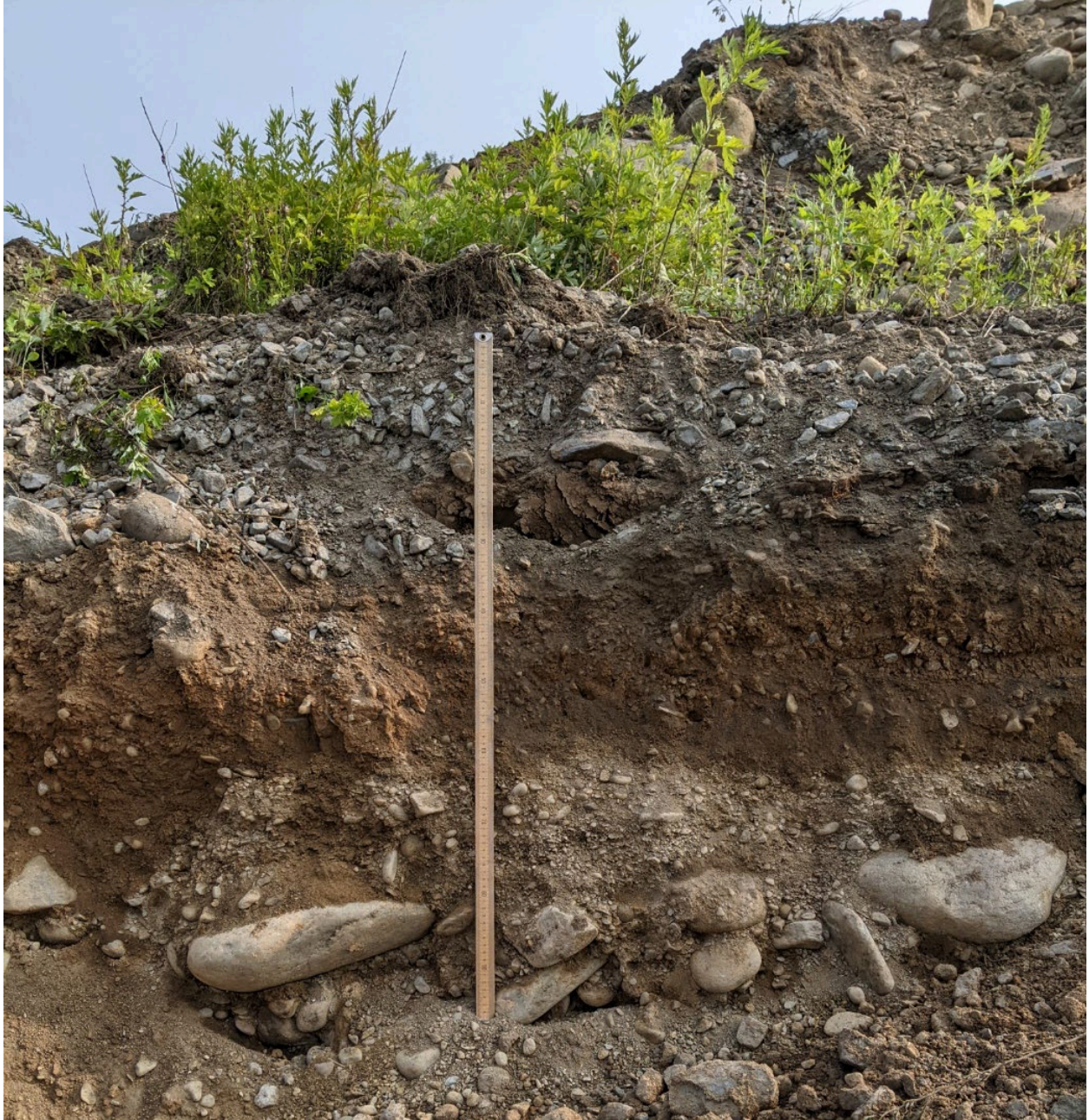
I-4A Medium sand to pebbles with few cobbles layer 0-0.75 m, sand and cobbles 0.75 to bottom (1 m). Layer fines upward. Layer is nearly horizontal (difficult to measure). Some imbrication of cobbles suggests eastward transport.
