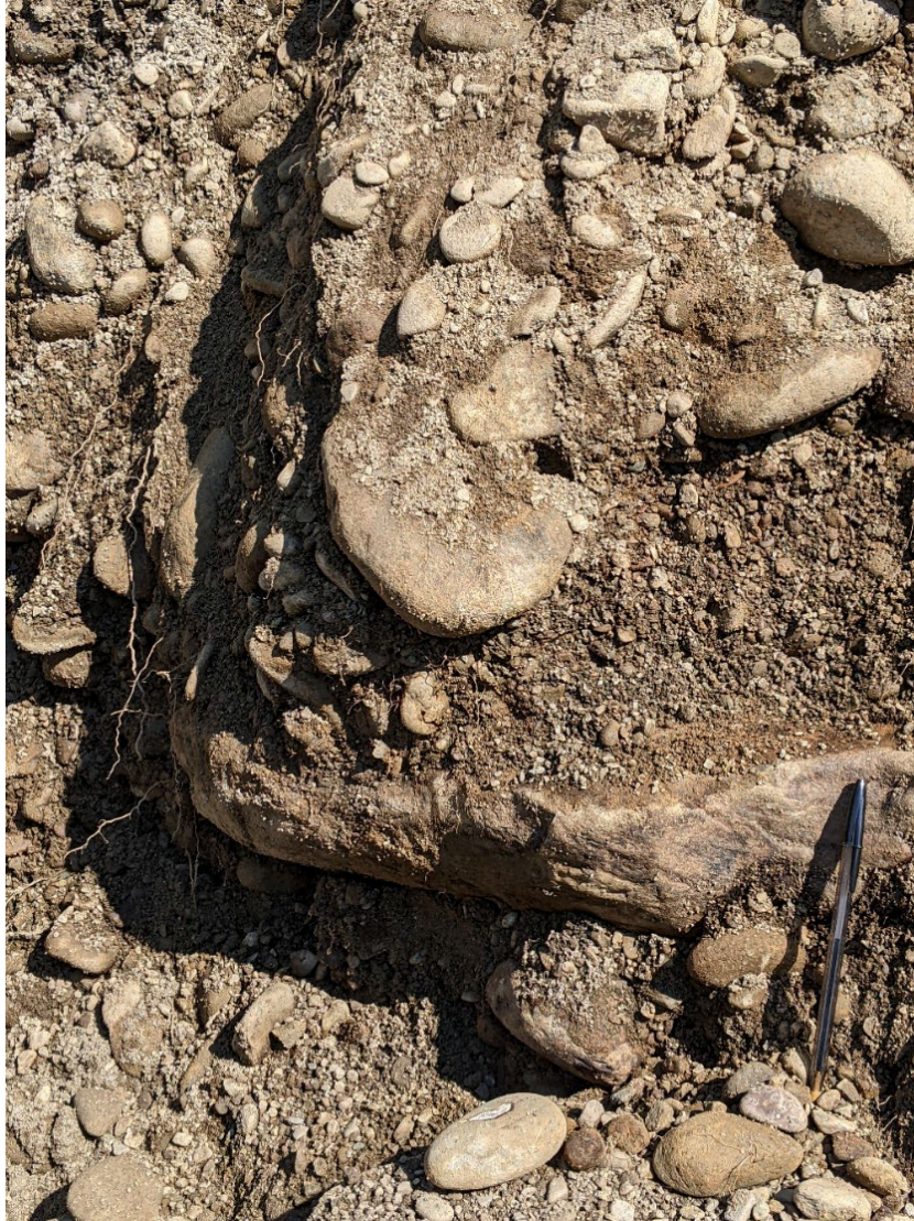
I-6A Rounded to well-rounded medium sand to cobbles. Poorly sorted, not graded. No bedding or sedimentary structures. Flat cobbles are approximately horizontal, weak imbrication in some cases. Apparent preferred long dimension orientations ( \sim 185^\circ ). Total depth 1.4 m.
