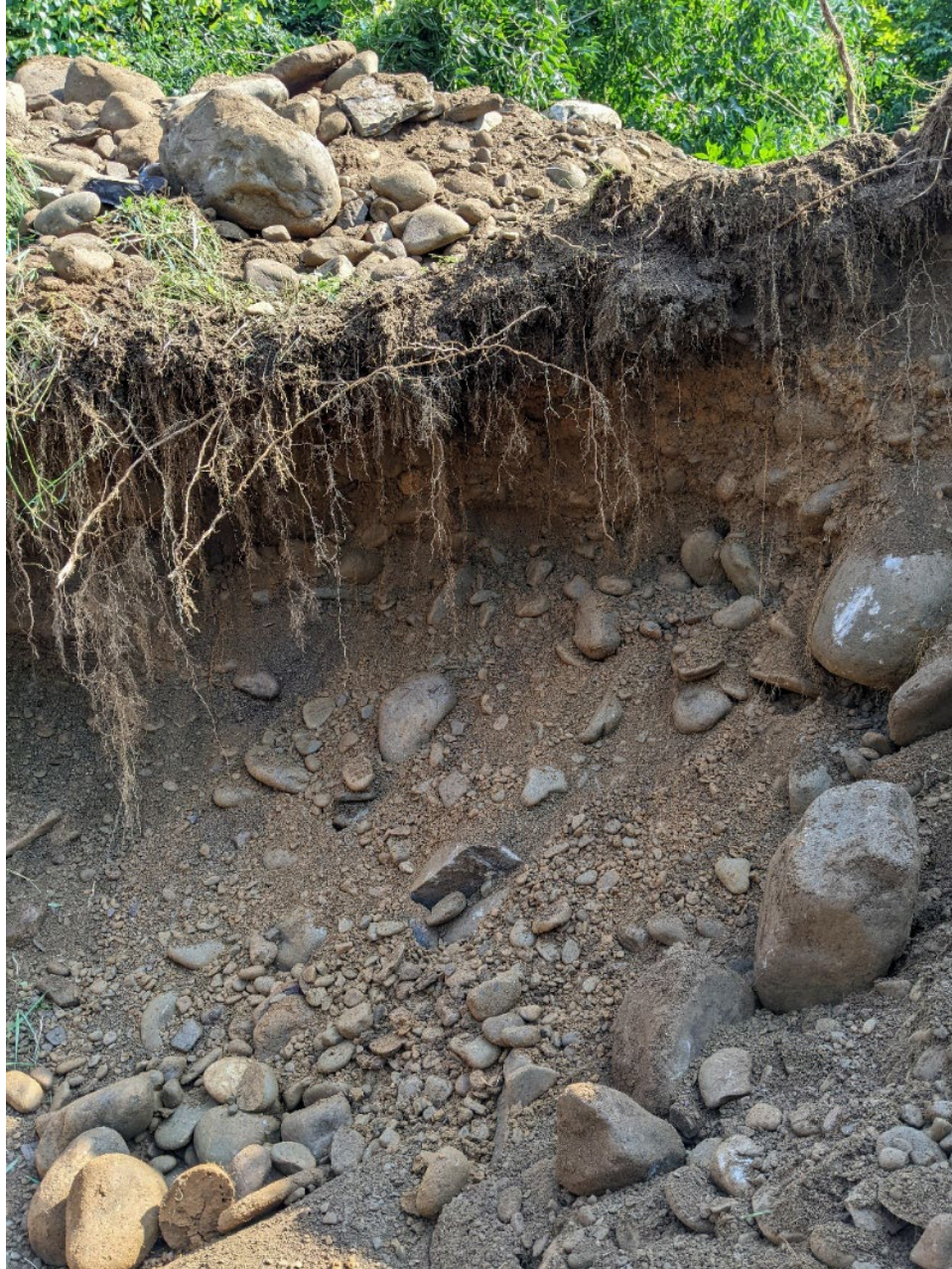
I-5A Medium sand to cobbles. Some fine sand and silt in B-horizon (to ~0.75 m). Total depth 1.5 m.
