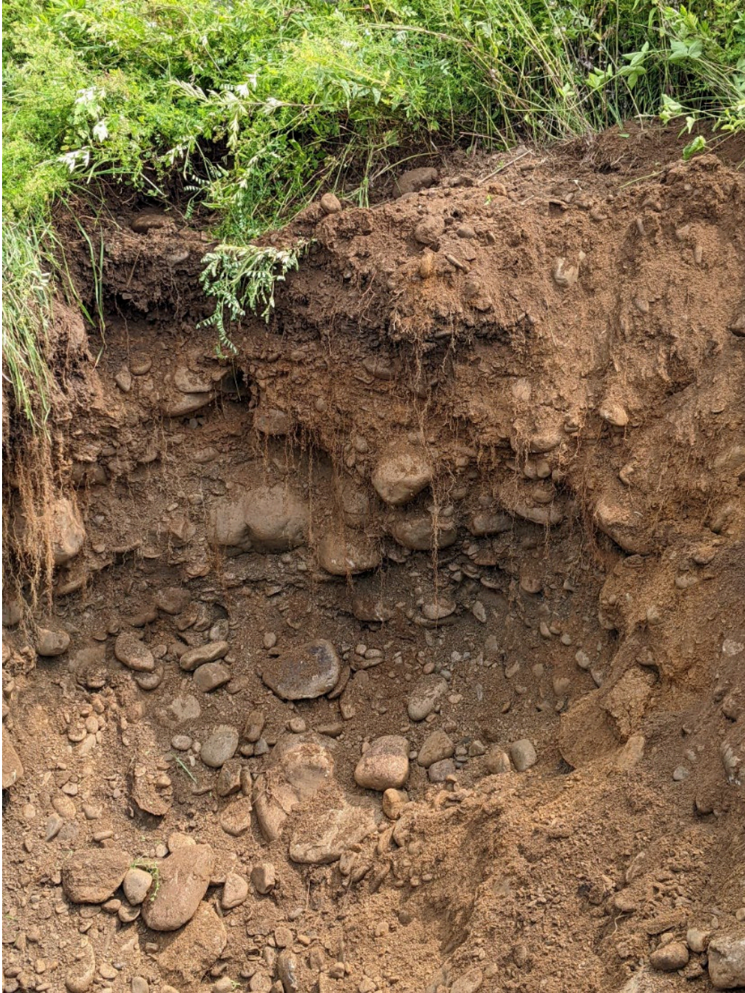
I-1A Medium sand to cobbles. Total depth 1.5 m.
