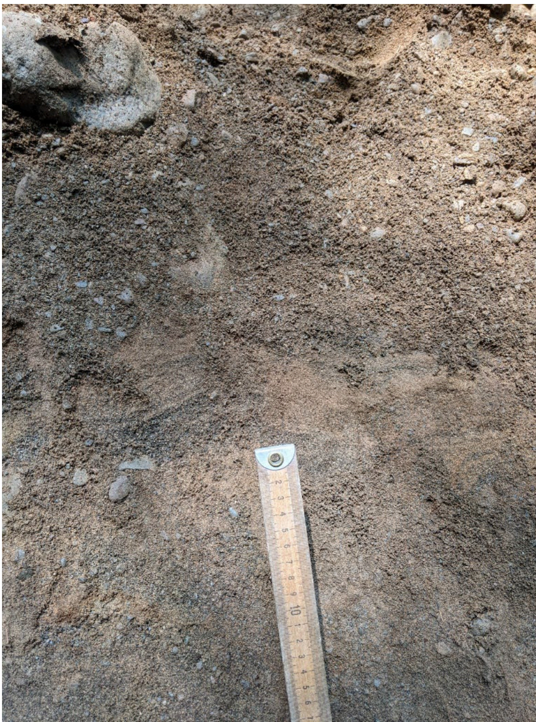
I-2A Medium sand with few granules and pebbles at 1.2 m. Possible small slump structure at top of meter stick.
