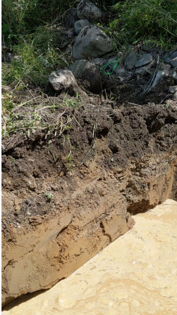
I-6E North wall of excavation adjacent to south side of pond. Fine sand 0 to 1.2 m. Water enters from pebble and cobble layer on west side at bottom. Large cobbles at surface. Small lens of sand and cobbles at 0.5 m in north wall. Water at ~0.7 m.
