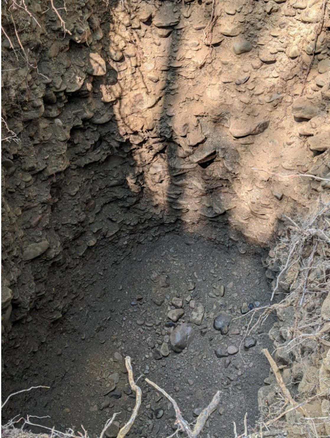
TP-16 Coarse sand to cobbles. Approximately horizontal alignment of cobbles. Slightly finer material near bottom. Total depth 5.2 m. Wet at bottom (no water).
