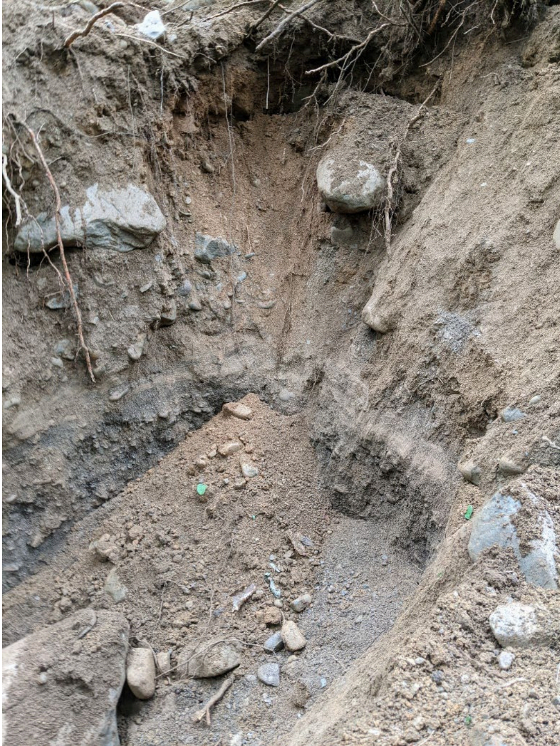
I-2A Medium sand to cobbles 0 to 1.2 m. Medium sand and medium sand to cobble layers at bottom. Layers dipping \sim 130^\circ , 23^\circ . Total depth 2.1 m.
