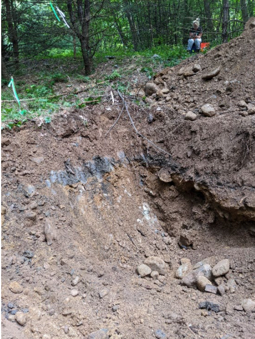
I2-B Old road. Buried A-horizon at 0.7 m. Medium sand to cobbles to 1.5 m.
