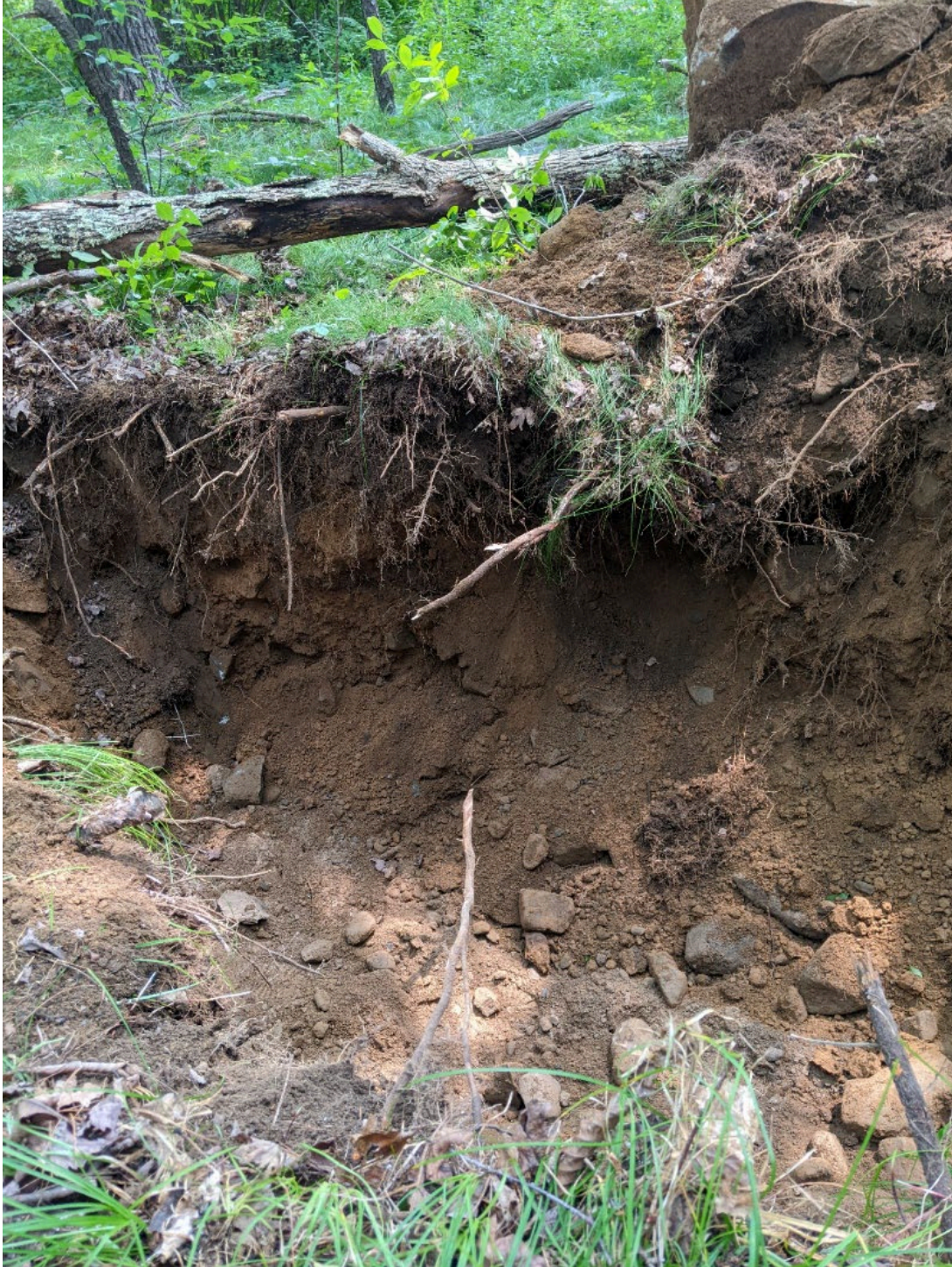
I-1B Medium sand to cobbles. Large cobbles at base (difficult excavation). Total depth 1.5 m.
