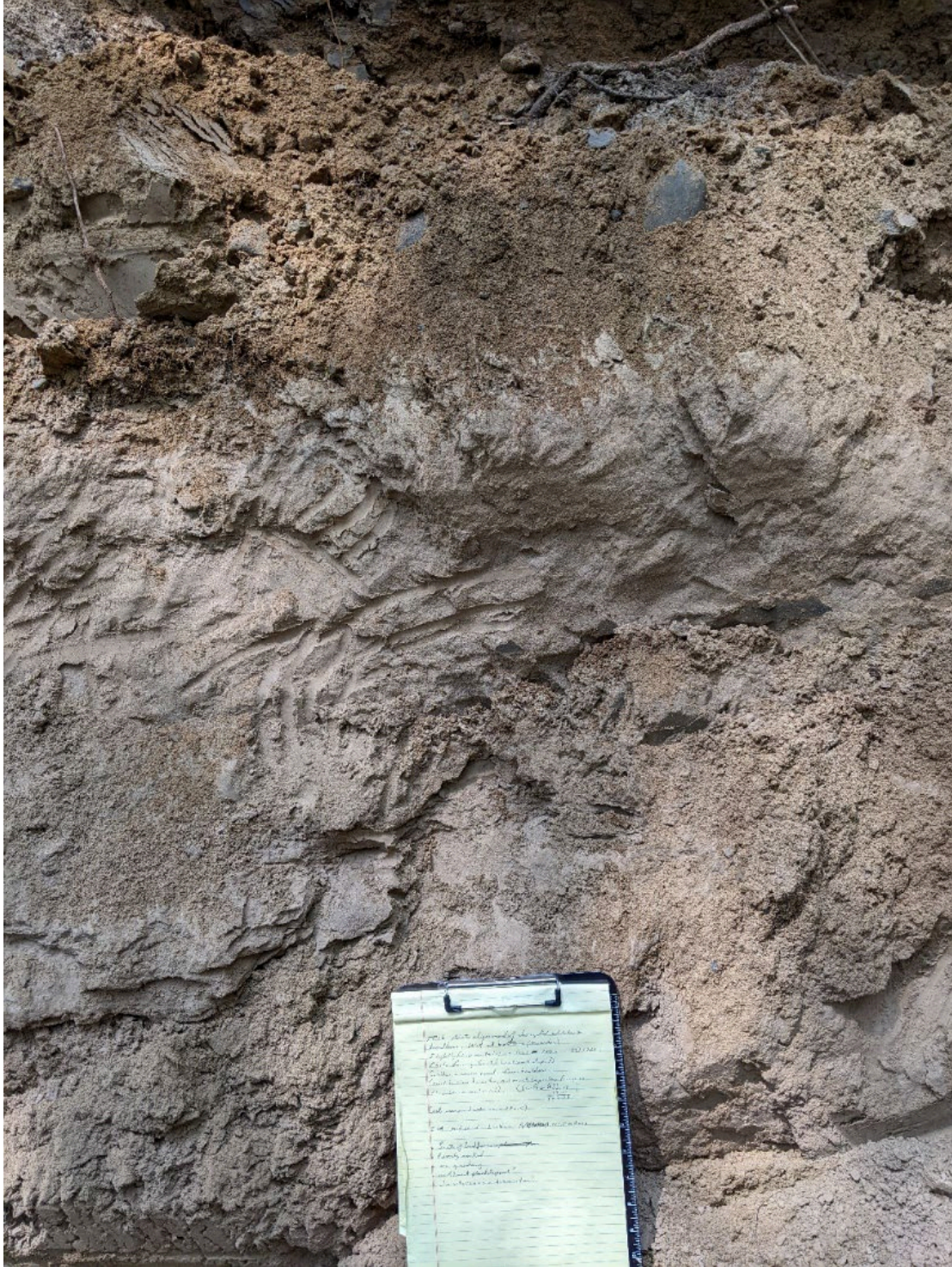
I-1C Fine sand. Platy structure in some areas. Predominantly massive. Thin planer beds are evident in some areas. No ripples or other sedimentary structures. (Relocated to 41.337739, -74.830601)
