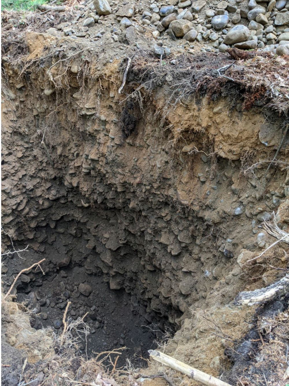
TP-15 Medium sand to cobbles 0-1 m. 1 m to 1.2 m coarse sand layer. 1.2 m to 4.9 m coarse sand and cobbles. Appears to be graded with large cobbles at bottom (up to ~0.5 m) to smaller cobbles to a depth of 1.2 m. Layers are approximately horizontal.
