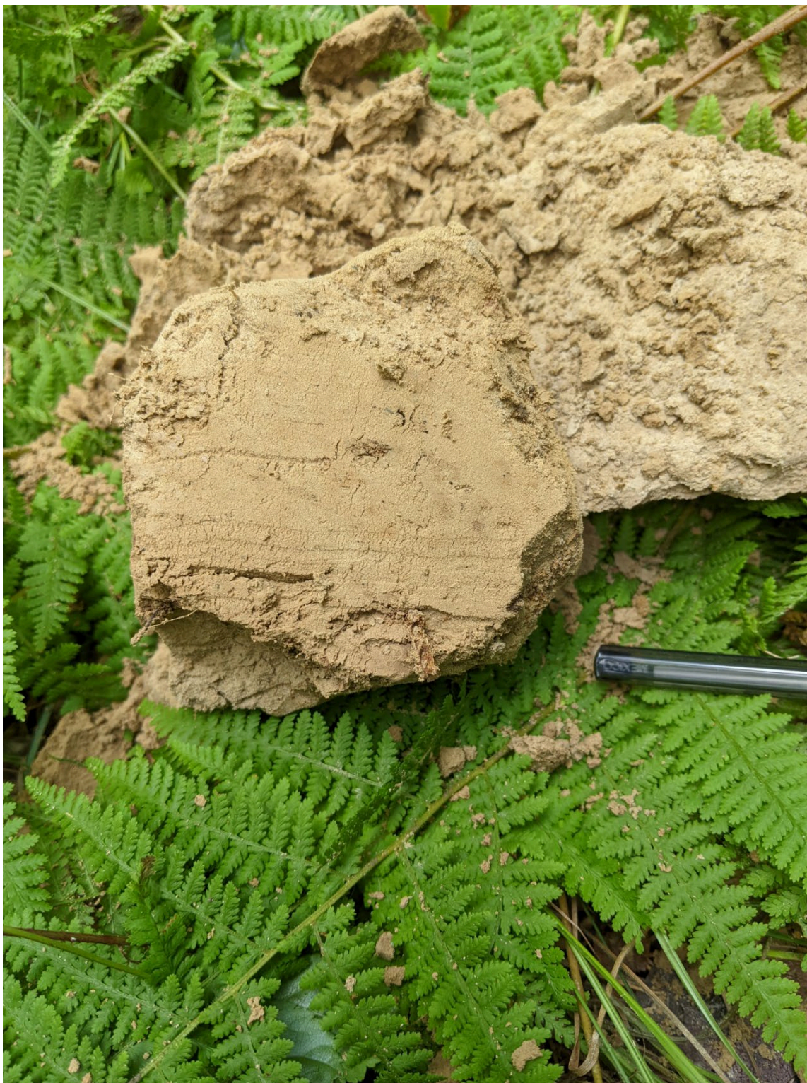
I-1C Fine sand showing thick lamination (~5 mm).
